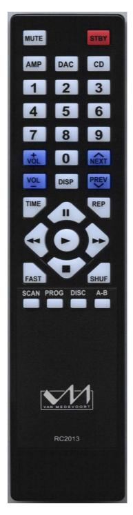
To switch the power ON or in Stand By mode STBY Mute the vM amplifier when connected **MUTE** Select first the device to control AMP **AMP** Use these buttons to select inputs 1~6 Skip button selects next input **NEXT** Skip button selects previous input PREV VOL+ Volume up on the connected vM amplifier VOL --
